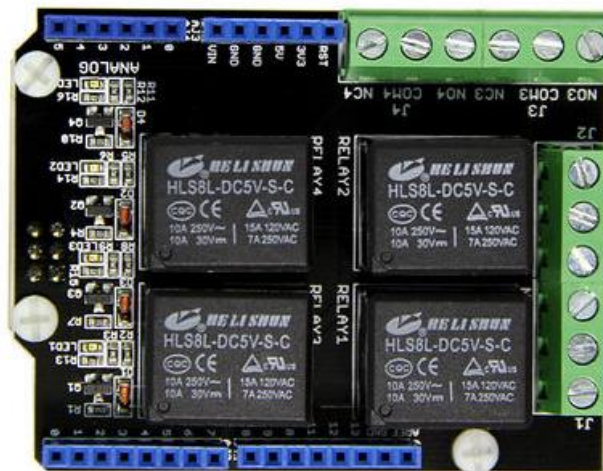
Figure 38. Example of an Arduino-compatible "shield" containing relays suitable for powering the linear motorized actuators from the 12 Vdc supply (e.g. SeeedStudio SLD01101P).
