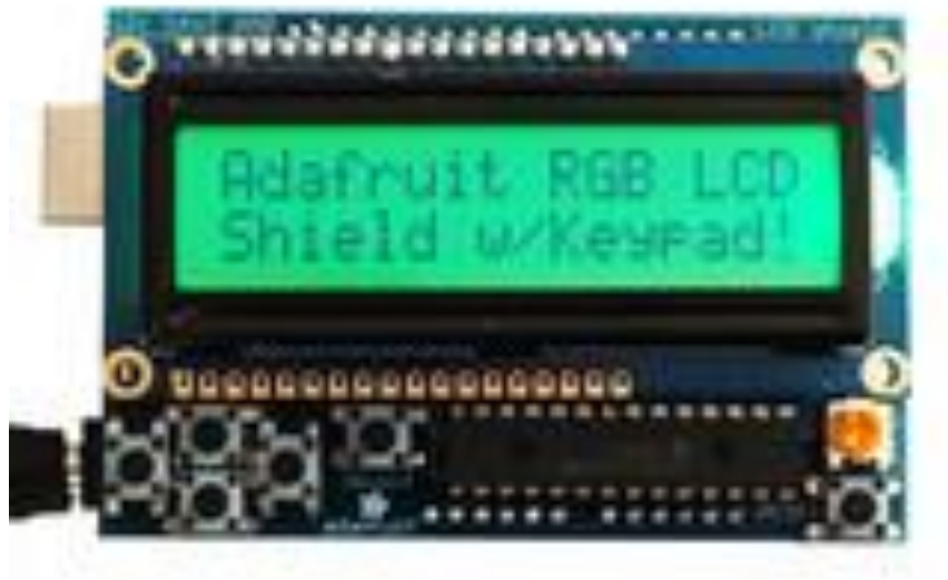
Figure 42. Example backlit-LCD PCBA assembly that is an Arduino "shield" for rapid integration (Adafruit Industries model MKAD44).
