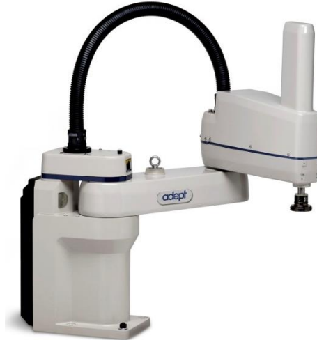
Figure 19. Example of industrial SCARA robot.
