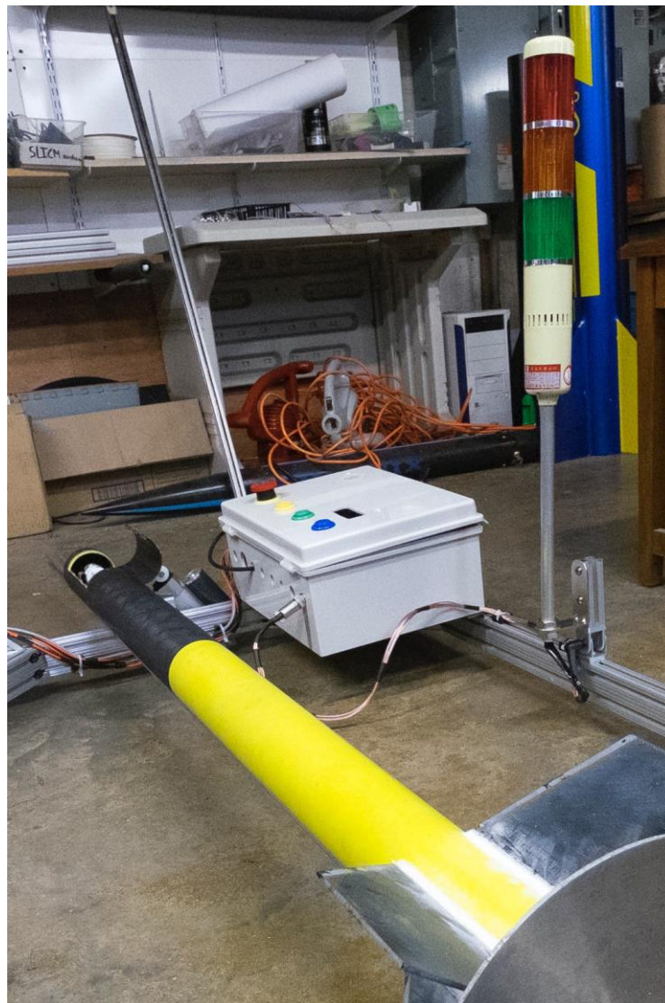
Figure 60. Status indicator beacon pole integrated with AGSE, control box, and full-scale launch vehicle.
