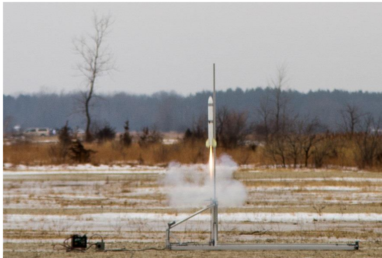
Figure 1: TARC rocket launched from AGSE to test AGSE's launch capability
