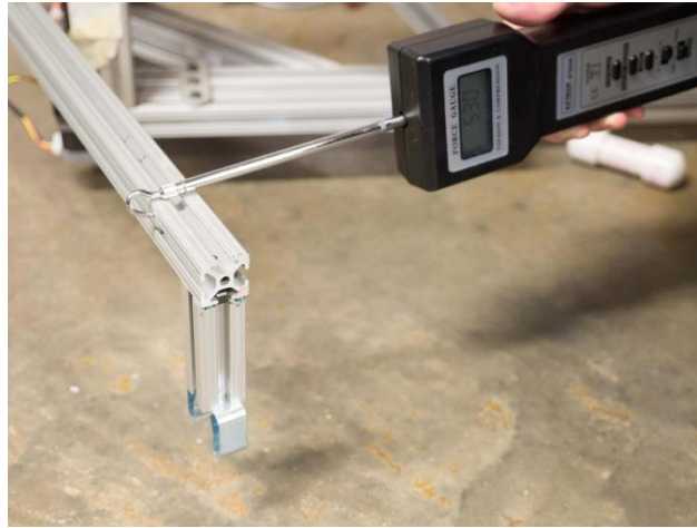
Figure 72: Measurement of SCARA arm peak force using load pull tester
