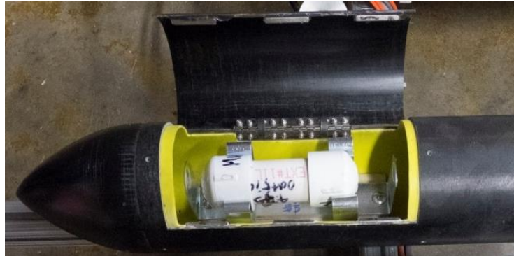
Figure 14: Payload compartment with a hinged door and a coupler (yellow) for reinforcement.
