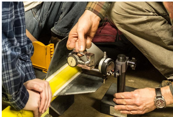
Figure 12: Fin deflection test setup
