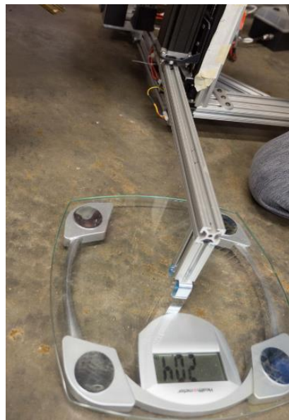
Figure 71: SCARA vertical stage load test
