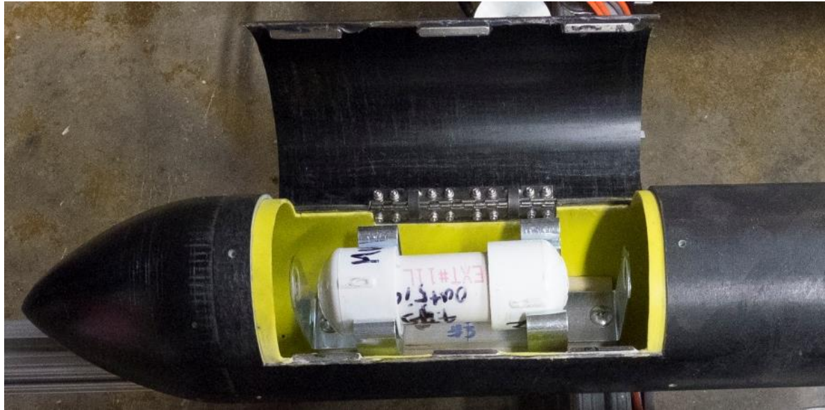
Figure 32. Image of completed full-scale payload retention bay showing door in open position (foam on door not present).
