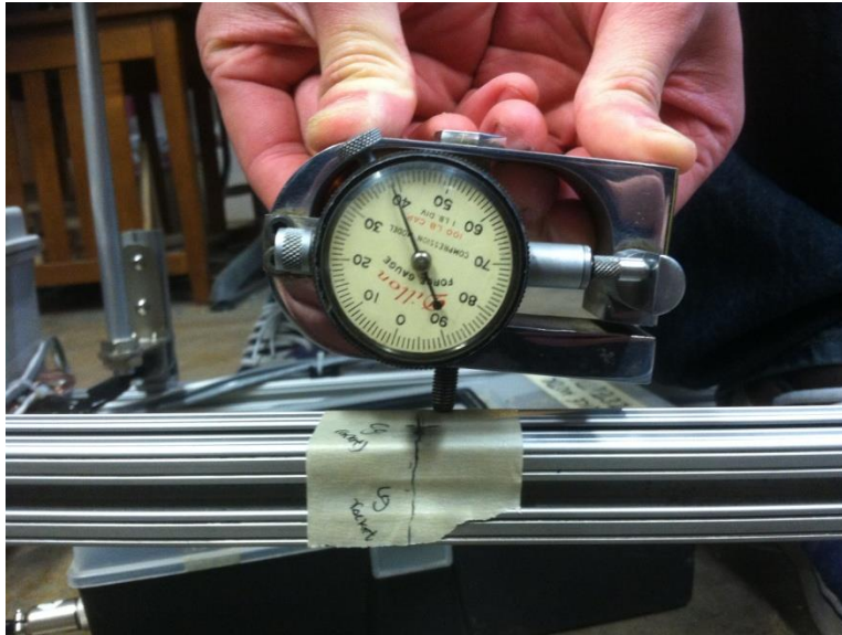
Figure 67. Rail load testing with calibrated dial gauge.
