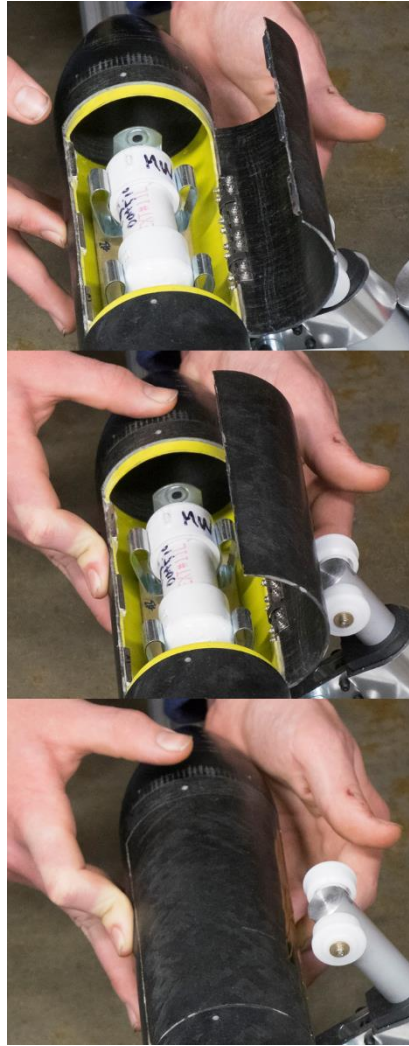
Figure 48: Real sequence of the door closing using the linear cylinder
