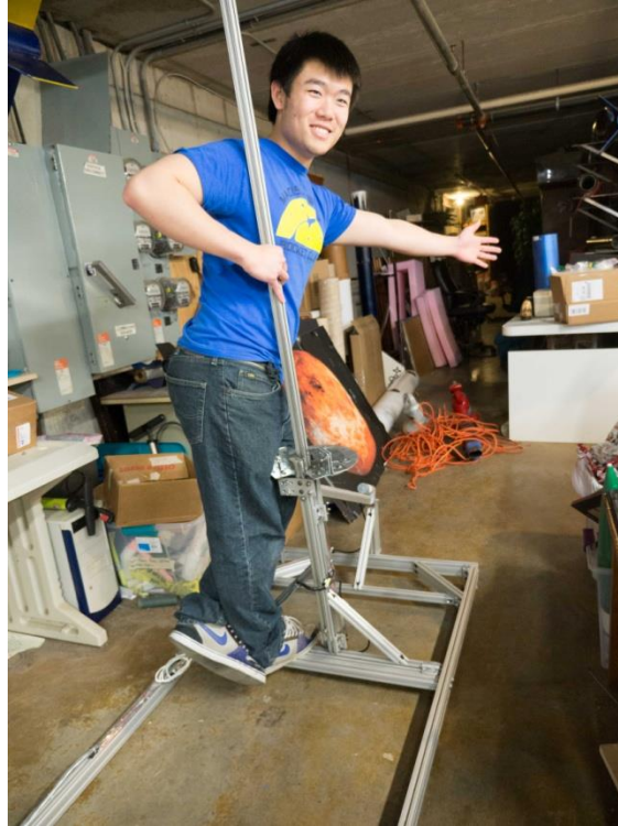
Figure 64. Deflection measurement testing of the AGSE structure using 10 pound ( top ) and 200 pound ( bottom ) loads
