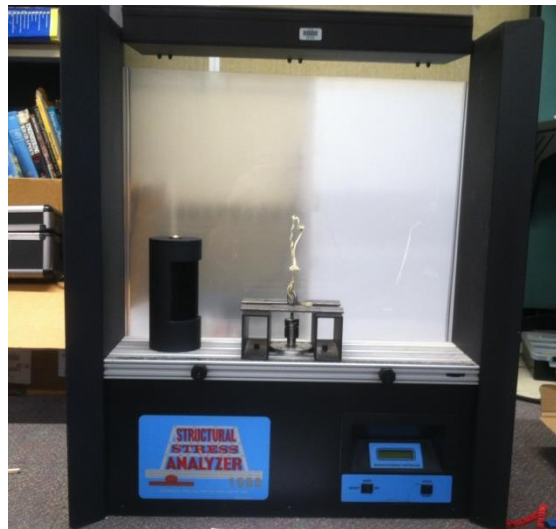
Figure 7: Structural stress analyzer used for tensile strength testing
