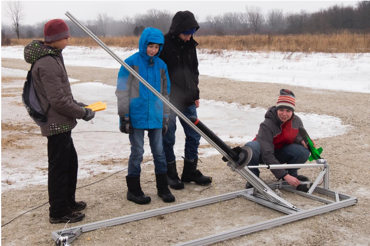
Figure 52. Freshman and sophomore members of Madison West SLI team testing the AGSE erection/launch system with F-class motor driven rockets.
