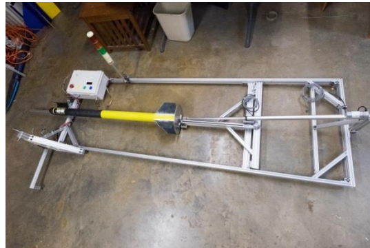
Figure 6: Full scale vehicle loaded on the AGSE. AGSE is now partly operational and fully launch capable.
