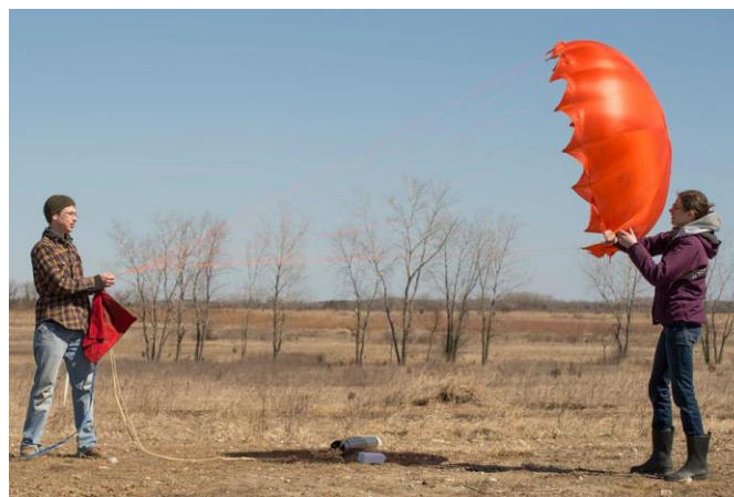
Figure 22: Parachute inflation test
