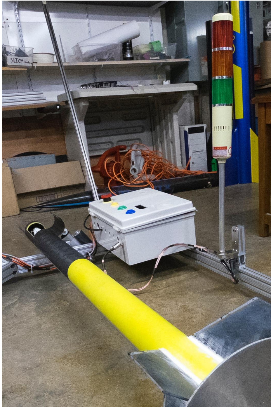
Figure 47. Status indicator beacon pole integrated with AGSE, control box, and full-scale launch vehicle.
