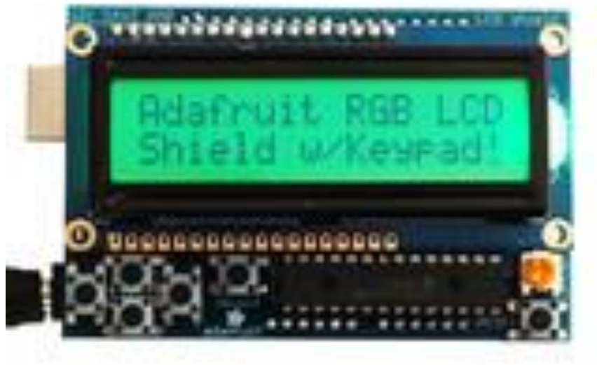
Figure 45. Example backlit-LCD PCBA assembly that is an Arduino "shield" for rapid integration (Adafruit Industries model MKAD44).
