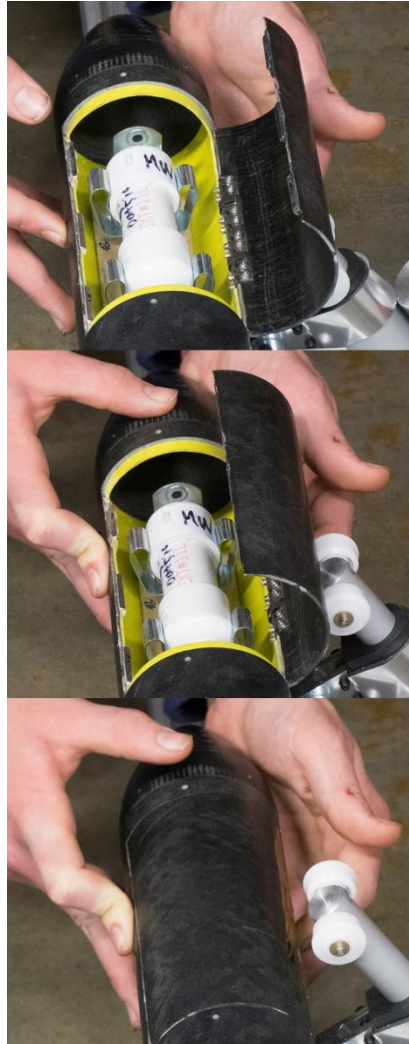
Figure 34 Real sequence of the door closing using the linear cylinder
