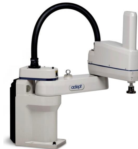
Figure 25. Example of industrial SCARA robot.
