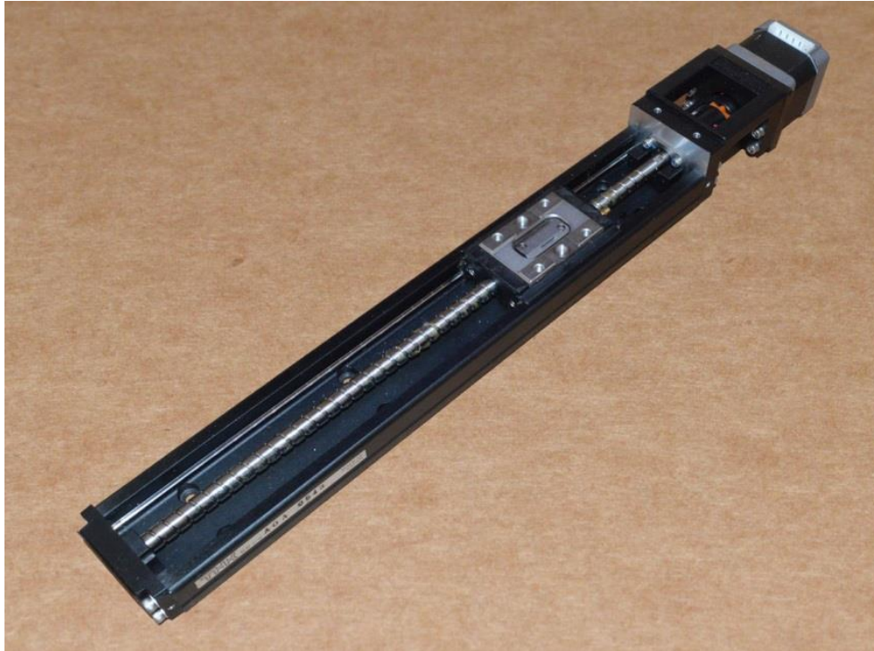
Figure 28. Compact linear stepper-motor driven vertical travel stage.
