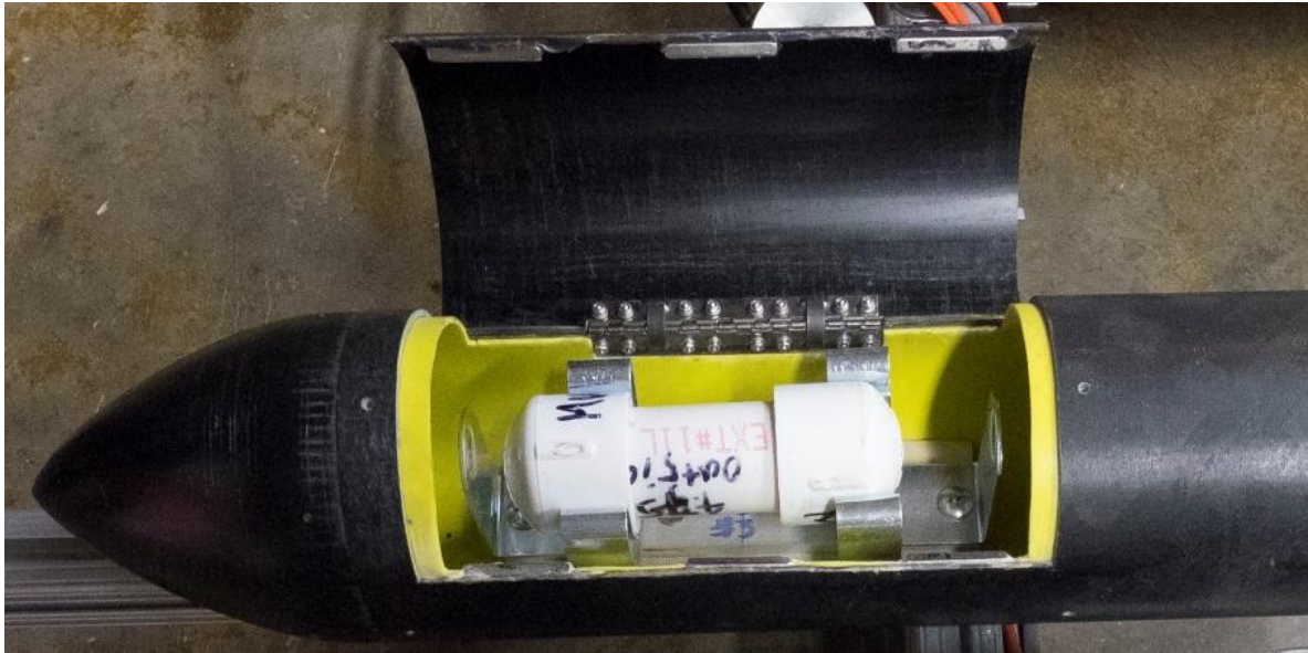
Figure 18. Image of completed full-scale payload retention bay showing door in open position (foam on door not present).
