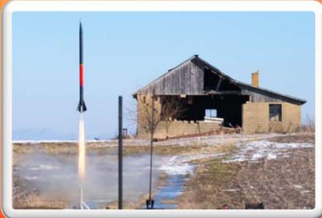
**FINAL:** J-class fiberglass rockets, 4500-5000g, to test AGSE robustness and launch capability under full intended load (1000N thrust). AGSE was tested up to 1700N thrust.
