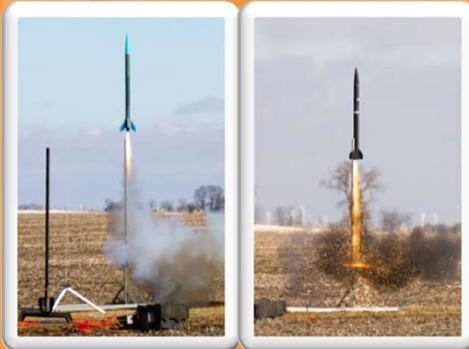
**ADVANCED:** H-class fiberglass/Blue Tube rockets, 1500g, to further test the blast deflector and to uncover possible stability problems
