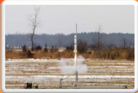
**INITIAL:** F-class TARC rockets, 650g, to verify rail and blast deflector functionality
