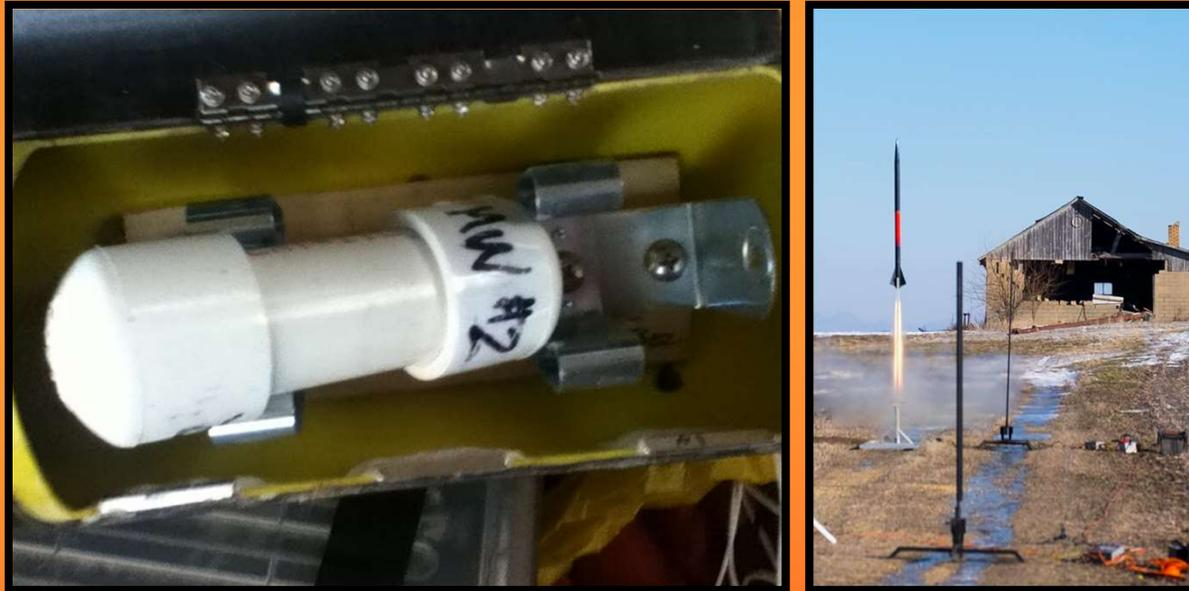
We have launched the payload compartment using auxiliary booster (Competitor kit) and CTI J1520VM motor. The payload door remained closed during flight and landing, however the payload has shifted forward and dislodged from the front clip. The shift forward indicates that the payload retention failed during deployment or landing, not during boost. A design modification will be made and the test will be repeated.
