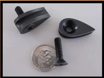
*Rail buttons* guide the rocket along the launch rail.
