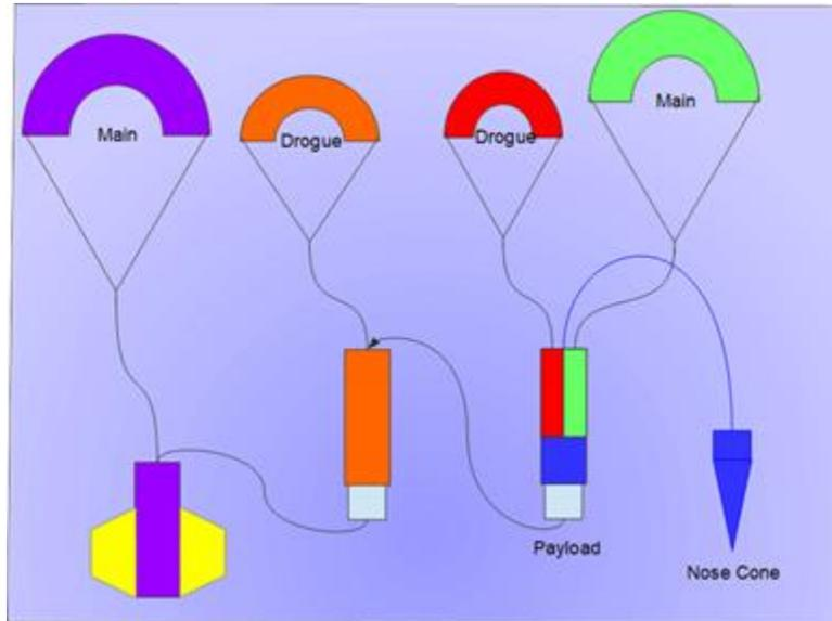
This image depicts our deployment system. At apogee, the vehicle separates into two untethered sections. The payload's drogue parachute is ejected directly below the nose cone, and the booster drogue is ejected out of the booster's upper tube, just below the camera array.
